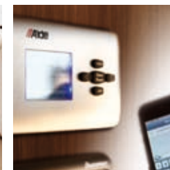
ALDE telemetric control to central heating (mobile phone connectivity via SMS)
